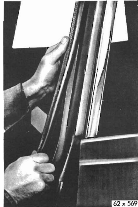
Fig. 10 - Removing or Installing door weatherstrip (typical view)
