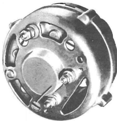
Fig. 24 - Alternator S.R. Head showing wire inserted to restrain brushes during assembly
