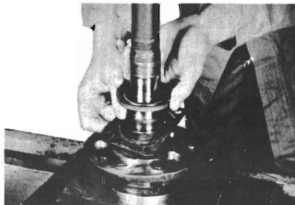
Fig. 12 - Positioning retainer plate and seal correctly on shaft.
