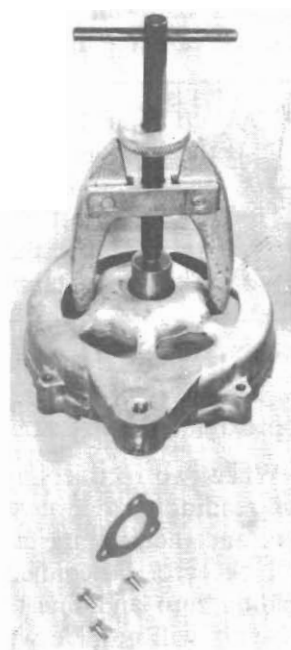
Fig. 16 - Pushing the Drive-End Bearing from the Housing using Press Adaptor
