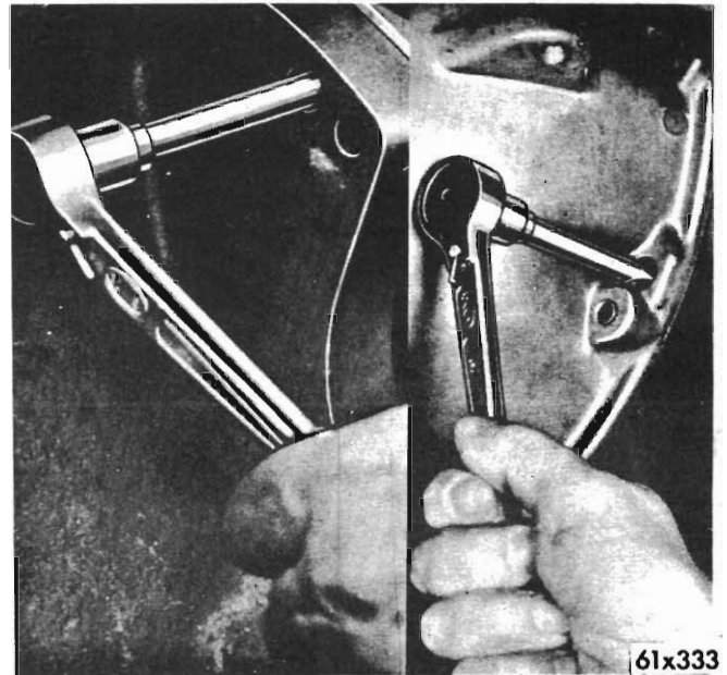
Fig. 4 - Adjusting offset dowels
