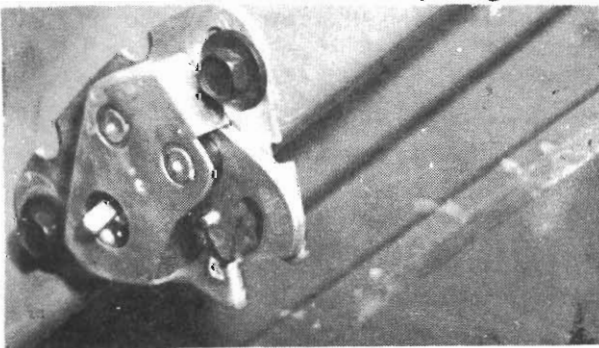
Fig. 22 - Deck lid lock adjustment
