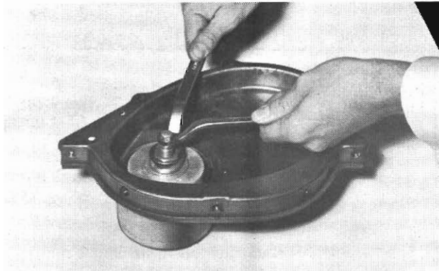
Fig. 29 - Installing new seal (Tool No. E9C57D)
