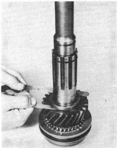
Fig. 23 - Checking end float; second speed gear
