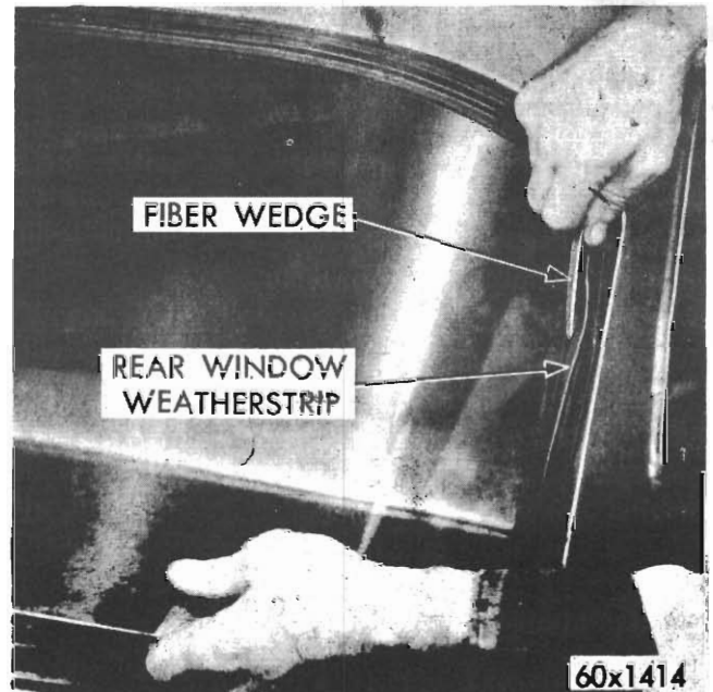
Fig. 37 - Removing or installing rear window glass (typical)
