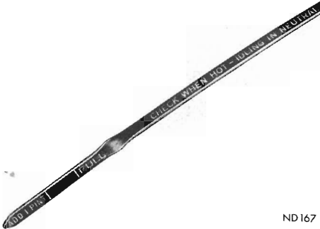
Fig. 14 - Automatic transmission dip stick markings
