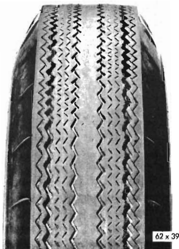
Fig. 12 - Over inflation wear
