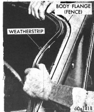
Fig. 33 - Removing or installing weatherstrip (typical view)
